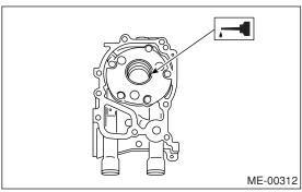
4) Position the oil pump, aligning the notched area with crankshaft, and push the oil pump straight.
