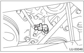
12) Remove the crank pulley by using ST. <Ref. to ME(H4DOTC)-39, REMOVAL, Crank Pulley.>
