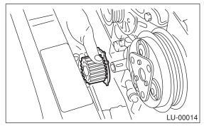
16) Remove the bolts which hold oil pump onto cylinder block.
