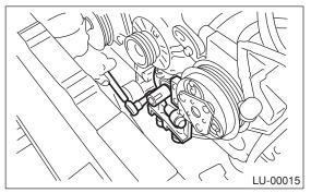
17) Remove the oil pump by using flat bladed screwdriver.
