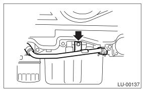
6) Remove the water pipe and hoses between oil cooler and water pump. (MT model)
