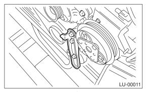
11) Remove the crankshaft position sensor.
