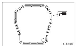
5) Tighten the bolts which install oil pan onto engine block.
