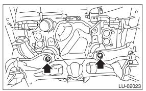
16) Remove the bolts which install oil pan on cylinder block with the engine raised up.
