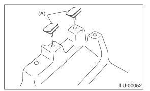
2) Install the baffle plate.
