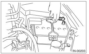
5) Disconnect the connector from mass airflow sensor.
