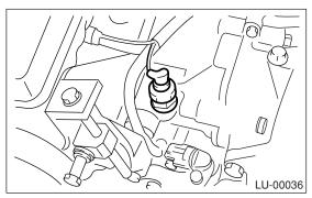
4) Install the generator to bracket. <Ref. to SC(H4SO)-20, INSTALLATION, Generator.> 5) Install the collector cover.
