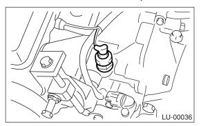
4) Remove the oil pressure switch.
