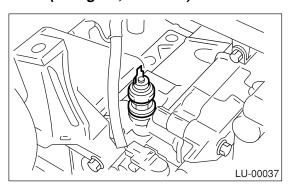
3) Connect the terminal to oil pressure switch.
