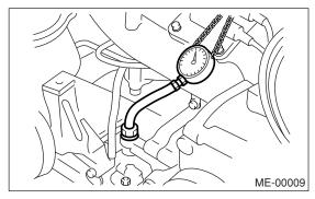
*Oil pressure (Standard): At 800 rpm 98 kPa (1.0 kgf/cm<sup>2</sup>, 14 psi) or more At 5,000 rpm*
