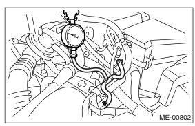
8) After connecting the pressure regulator vacuum hose, measure the fuel pressure.
