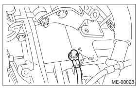
(3) Generator connector, terminal and A/C compressor connector
