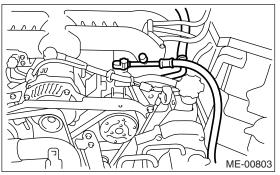
11) Repair the air intake system.
