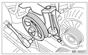
(2) Connect the power steering switch connector.
