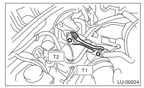
7) Remove the ST from converter case. (AT model) NOTE:
