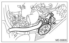
(4) Place the power steering pump on the right side wheel apron.
