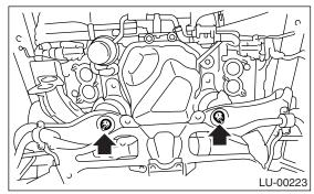
14) Install the center exhaust pipe.
