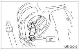
(3) Remove the bolts which hold upper side of the transmission to engine.
