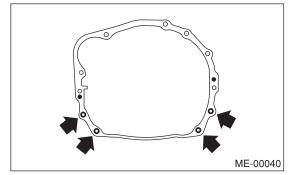
13) Tighten the nuts which install the front cushion rubber onto crossmember.
