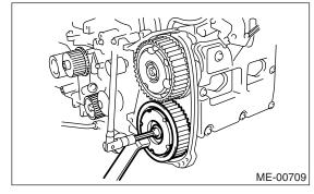
ST 499977500 CAMSHAFT SPROCKET WRENCH
