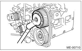
2) Install the timing belt. <Ref. to ME(H4DOTC)-42, INSTALLATION, Timing Belt.>
