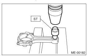
(3) Make two 3 mm (0.12 in) holes in bushing. Ream the inside of bushing.
