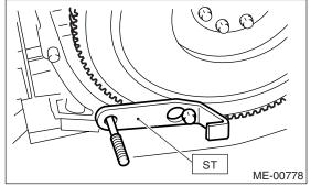
12) Remove the drive plate. (AT model) To lock crankshaft, use ST.
