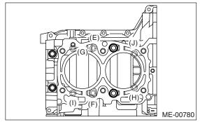
11) Tighten the 8 mm and 6 mm cylinder block connecting bolts on LH side (A — H) in alphabetical sequence.
