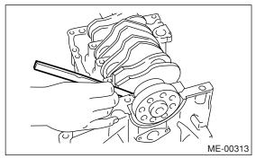
5) Inspect individual crankshaft bearings for signs of flaking, seizure, melting, and wear.
