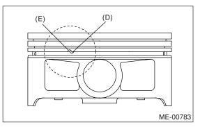
17) Position the expander gap at  $180^{\circ}$  on the reverse side of (C) that shown (F) in the figure.
