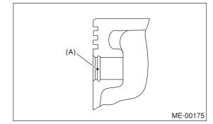
5) Check the piston pin snap ring for distortion, cracks and wear.
