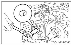
26) Rotate the crankshaft to bring #1 and #2 pistons to bottom dead center position, then remove the piston snap ring through service hole of #1 and #2 cylinders.
