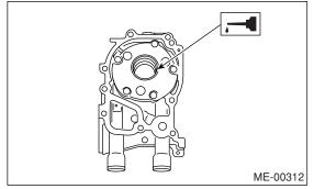
(4) Install the oil pump on cylinder block. Be careful not to damage the oil seal during installation.
