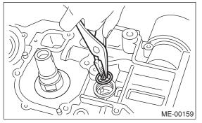
(4) Apply liquid gasket around the service hole plug.
