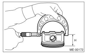
5) Calculate the clearance between cylinder and piston.
