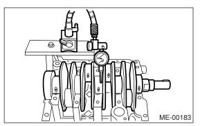
3) Inspect the crank journal and crank pin for wear. If they are not within the specifications, replace the bearing with a suitable (undersize) one, and replace or recondition crankshaft as necessary. When grinding the crank journal or crank pin, finish them to the specified dimensions according to the undersize bearing to be used. Crank pin:
