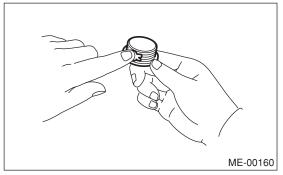
(5) Install the service hole plug and gasket.
