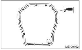
27) Apply liquid gasket to the mating surfaces and threaded portion of bolt (A) as shown in the figure, and install the oil separator cover.
