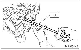
28) Similarly remove the piston pins from #3 and #4 pistons.
