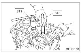
(2) Apply a coat of engine oil to piston pin, and insert the piston pin into piston and connecting rod through service hole.
