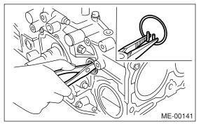
27) Draw out the piston pins from #1 and #2 pistons using ST.
