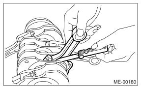
4) Inspect the connecting rod bearing for scar, peeling, seizure, melting, wear, etc.
