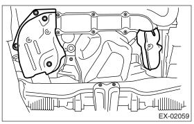
5) Remove the nuts which hold front exhaust pipe assembly to turbocharger joint pipe.
