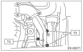
6) Install the exhaust manifold lower cover (RH) and the exhaust manifold lower cover (LH).
