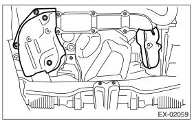
7) Install the front oxygen (A/F) sensor. <Ref. to FU(H4DOTC)-35, INSTALLATION, Front Oxygen (A/F) Sensor.>
