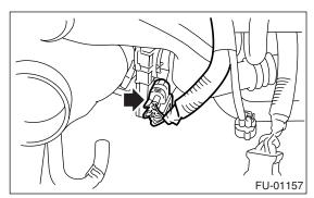
5) Disconnect the engine coolant hose from throttle body.
