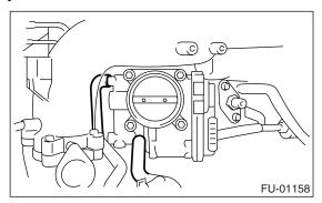
6) Remove the bolts which secure throttle body to intake manifold.
