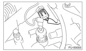
6) Remove the engine coolant temperature sensor.
