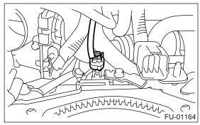
5) Remove the knock sensor from cylinder block.
