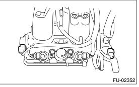
6) Remove the fuel injector. <Ref. to FU(H4DOTC)-29, REMOVAL, Fuel Injector.>
