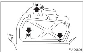
5) Remove the nut and bolt which hold the ECM to bracket.
