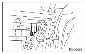
4) Disconnect the connector from main relay.
