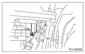
4) Disconnect the connector from electronic throttle control relay.
