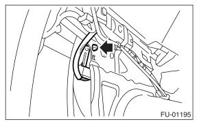
4) Disconnect the connector from fuel pump control unit.
