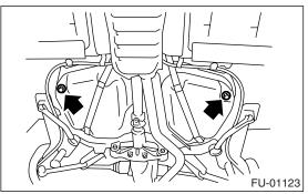
7) Tighten the fuel drain plug. NOTE:
