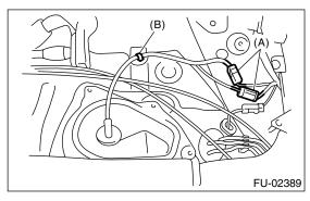
26) Connect the connector to fuel pump.
