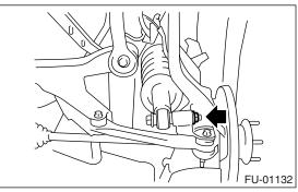
7) Tighten the bolts which install the parking brake cable clamp.
