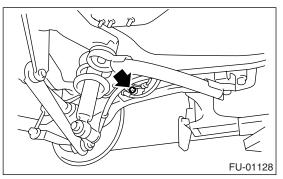
17) Remove the rear brake caliper and tie it to the vehicle body side.
