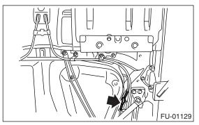
9) Install the heat shield cover.
