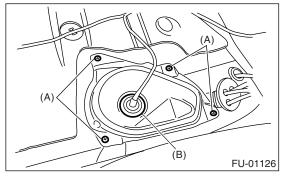
9) Disconnect the connector (A) from fuel sub level sensor.
