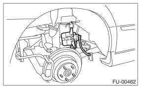
18) Remove the parking brake cable from parking brake assembly. <Ref. to PB-6, REMOVAL, Parking Brake Assembly (Rear Disc Brake).>
