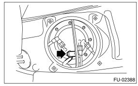
27) Install the service hole cover of fuel pump.
