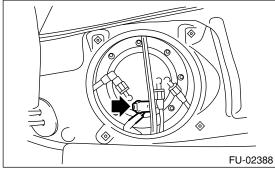
7) Remove the connector (A) and clips (B).
