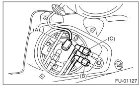
24) Install the service hole cover of fuel sub level sensor.
