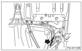
24) Remove the bolts which install the parking brake cable clamp.
