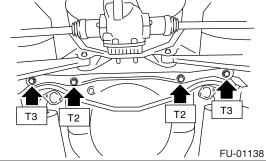
(3) Tighten the bolts which install the rear shock absorber to rear suspension arm. <Ref. to RS-11, INSTALLATION, Rear Arm.>
