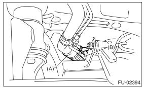
29) Support the fuel tank with transmission jack, remove the bolts from fuel tank bands, and dismount the fuel tank from vehicle.
