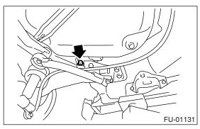
8) Connect the connector to rear ABS wheel speed sensor.
