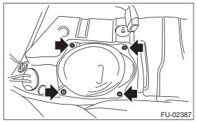
6) Disconnect the connector from fuel pump.
