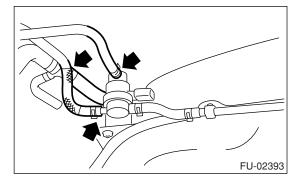
28) Disconnect the fuel filler hoses (A) and evaporation hoses (B).
