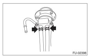
2) Remove the nut which holds the evaporation pipe assembly to fuel filler pipe.
