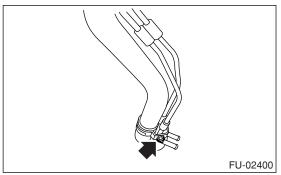
3) Remove the shut valve from fuel filler pipe. <Ref. to EC(H4DOTC)-15, REMOVAL, Shut Valve.>
