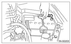
4) Remove the screws which secure the packing.
