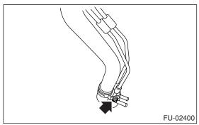
3) Connect the evaporation hose to shut valve.
