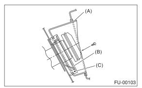
4) Correctly insert the fuel filler hose (A) and evaporation hose (B) to specified position, and then tighten the clamp.
