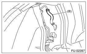
12) Remove the fuel filler pipe to under side of the vehicle.
