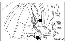
11) Loosen the clamp and disconnect the fuel filler hose (A) and evaporation hose (B).
