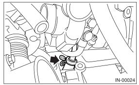
15) Take out the turbocharger from engine compartment.
