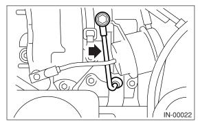
13) Remove the turbocharger bracket.
