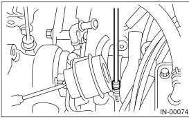
11) Remove the bolt which secures bracket of oil pipe to turbocharger.
