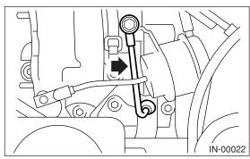
4) Install the joint pipe to turbocharger.
