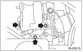
5) Install the turbocharger bracket.
