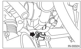
2) Install the turbocharger to intake duct.
