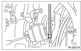
3) Install the oil pipe to turbocharger.
