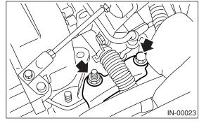
14) Disconnect the oil outlet hose from pipe.
