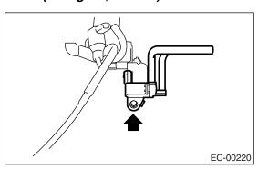
NOTE: Connect the evaporation hose as shown in the figure.
