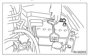
3) Remove the solenoid valve bracket assembly from intake manifold.
