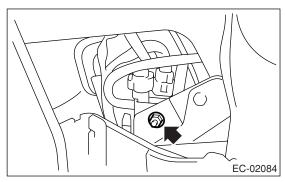
NOTE: Replace the fuel tank pressure sensor and fuel tank sensor control valve as a unit.
