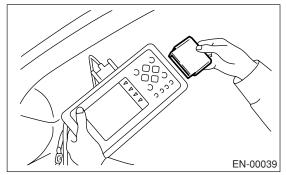
6) Connect the test mode connector (A) at the lower portion of glove box.
