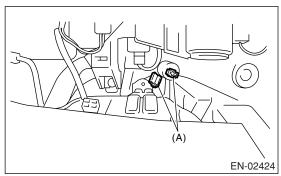
4) Connect the OBD-II general scan tool to its data link connector in the lower portion of instrument panel (on the driver's side).
