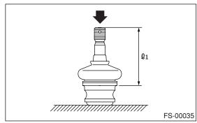
(2) With 686 N (70 kgf, 154 lb) loaded in direction shown in the figure, measure the dimension  $\varrho_2$ .
