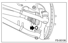
5) Remove the nut securing the front arm to crossmember. (Do not remove the bolt.)
