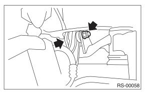
4) Remove the bolts which secure the upper link to rear arm, and then remove the upper link.
