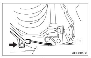
4) Remove the rear ABS wheel speed sensor from rear arm.
