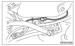
3) Remove the sensor harness bracket from rear arm.
