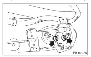
6) Remove the inner cable end from equalizer.
