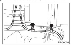
12) Remove the cable assembly.
