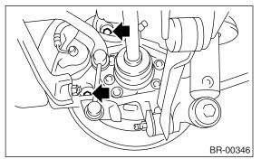
3) Suspend the brake caliper assembly so that the hose is not stretched.
