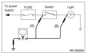
4) With the test set-up held as it is, turn the switch ON. The voltmeter will indicate a voltage and, at the same time, the light will come on.
