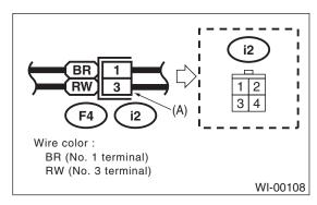
• In the wiring diagram, connectors which have no terminal number refer to one-pole types. Sketches of these connectors are omitted intentionally.
