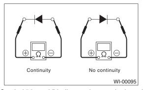
3) Symbol "○ — ○" indicates that continuity exists between two points or terminals. For example, when a switch position is at "3", continuity exists among terminals 1, 3 and 6, as shown in the table below.
