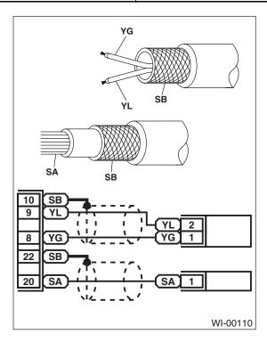
• The wire color code, which consists of two letters (or three letters including Br or Lg), indicates the standard color (base color of the wire covering) by its first letter and the stripe marking by its second letter.
