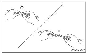
5) Some connectors are provided with a lock. One type of such a connector is disconnected by pushing the lock, and the other, by moving the lock up. In either type the lock shape must be identified before attempting to disconnect the connector.
