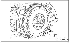
2) Tighten the flywheel mounting bolts to specified torque.
