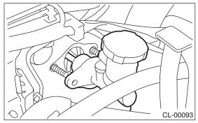
7) Remove the bolts and nuts which secure brake pedal and clutch pedal, and remove the pedal assembly.
