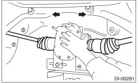
7) Adjust the transmission jack, if necessary, and insert the rear differential stud bolt into rear crossmember bushing properly.
