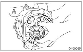
7) When replacing the side bearing, remove the bearing cup from side bearing retainer using ST. ST 398527700 PULLER ASSY
