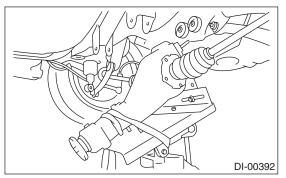
18) Pull out the axle shaft from rear differential. NOTE:
