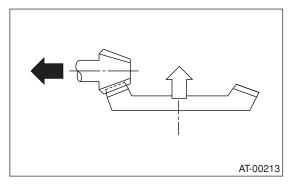
• Toe contact (inside end contact) Checking item: Contact areas is small Contact pattern
