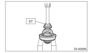
13) Press-fit the side bearing cone to the side bearing retainer using ST.
