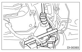
8) After inserting the rear differential stud bolt into rear crossmember bushing, lift up the transmission jack and align the rear differential with its own position.
