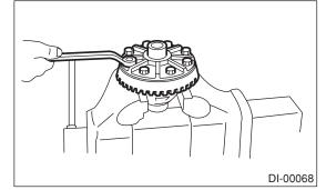
12) Press the side bearing into differential case using ST.
