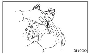
16) Check the hypoid driven gear runout on its back surface, and make sure that pinion and hypoid driven gear rotates smoothly.
