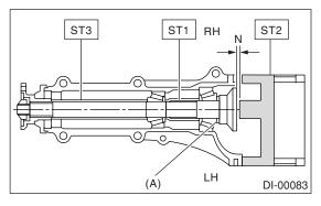
(A) Pinion height adjusting washer
