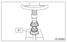
4) Insert the drive pinion into differential carrier, install the selected bearing preload adjusting collar and washer.
