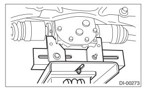
14) Secure the rear differential using band.
