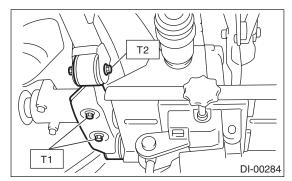
12) Tighten the self-locking nut.
