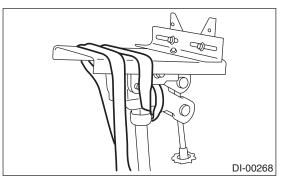
10) Loosen the self-locking nuts which hold the rear differential to rear crossmember.
