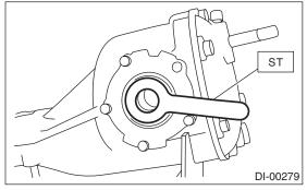
4) Insert the spline shaft until the spline portion comes inside the side oil seal.
