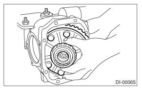
(3) Install the side bearing retainer shims to retainers RH and LH from which they were removed.
