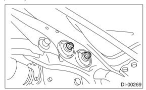
10) Remove the band from rear differential. Lift up the rear differential until the rear differential is separated from the transmission jack.
