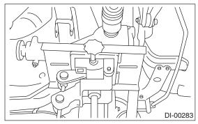
9) Tighten the rear crossmember self-locking nut temporarily.
