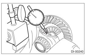
(2) Adjust the side gear backlash as specified by selecting side gear thrust washer.
