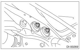
11) Remove the DOJ of rear drive shaft from rear differential using ST.
