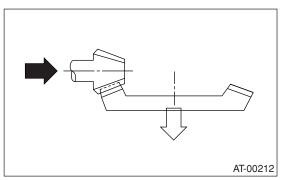
18) If proper tooth contact is not obtained, once again adjust the drive pinion height by changing RH and LH side bearing retainer shims and the hypoid gear backlash.
