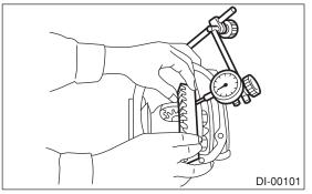
17) Checking and adjusting the tooth contact of hypoid driven gear
