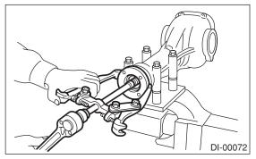
14) Press the end of drive pinion shaft and extract it together with rear bearing cone, pinion height adjusting washer and washer.
