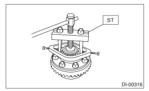
9) Remove the hypoid driven gear by loosening hypoid driven gear bolts.
