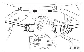
7) Adjust the transmission jack, if necessary, and insert the rear differential stud bolt into rear cross-member bushing properly.
