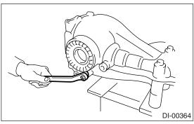
(5) Measure the hypoid driven gear-to-drive pinion backlash. Set the magnet base on differential carrier. Align the contact point of dial gauge with tooth face of hypoid driven gear, and move hypoid driven gear while holding drive pinion still. Read the value indicated on dial gauge.
