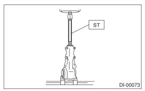
17) Remove the rear bearing cone from drive pinion by supporting the cone with ST.
