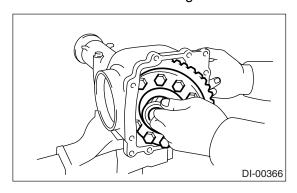
7) Remove the bearing race from holder RH and LH with ST1 and press.
