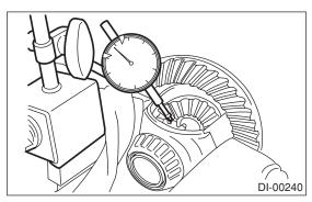
(2) Adjust the side gear backlash as specified by selecting side gear thrust washer.
