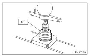
(3) Install the differential assembly into differential carrier in the reverse order of disassembly.
