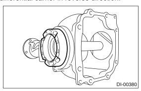
(3) Measure the clearance N between the end of ST2 and the end surface of ST1 by using a thickness gauge.
