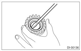
10) Extract the bearing cone with ST1 and ST2.
