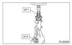
9) Install a new self-locking nut, and secure the companion flange using ST, and tighten the nut. ST 498427200 FLANGE WRENCH
