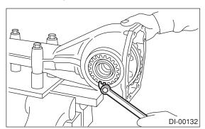
17) Recheck the hypoid driven gear to pinion backlash.
