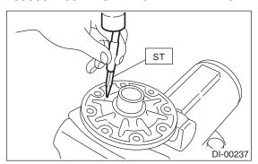
13) Draw out the pinion mate shaft and remove pinion mate gears, side gears and thrust washers.
