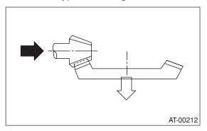
19) If proper tooth contact is not obtained, once again adjust the drive pinion height and the differential side bearing preload (already mentioned) and the hypoid gear backlash.
