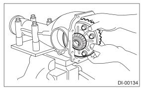
8) Remove the bearing race from holder RH and LH with ST1 and ST2.
