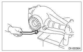
16) Recheck the hypoid driven gear to pinion backlash.
