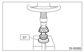
4) Insert the drive pinion into differential carrier, install the selected bearing preload adjusting collar and washer.
