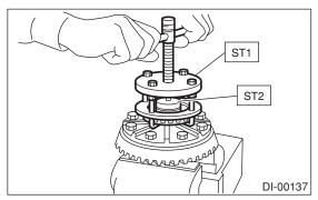
11) Remove the hypoid driven gear by loosening hypoid driven gear bolts.
