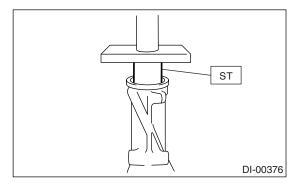
(3) Insert the front bearing cone.
