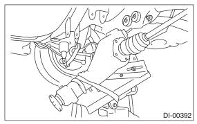
20) Pull out the axle shaft from rear differential.
