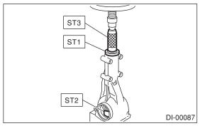
6) Insert the collar, then press-fit the pilot bearing with ST1 and ST2.
