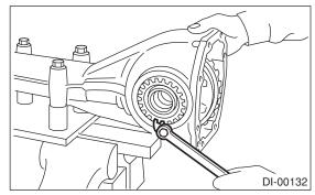
(5) Measure the hypoid driven gear-to-drive pinion backlash. Set the magnet base on differential carrier. Align the contact point of dial gauge with tooth face of hypoid driven gear, and move hypoid driven gear while holding drive pinion still. Read the value indicated on dial gauge.
