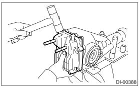
4) Remove the lock plate RH and LH.
