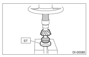
4) Insert the drive pinion into differential carrier, install the previously selected bearing preload adjusting collar and washer.
