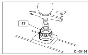
(2) Install the bearing race into holder RH and LH.
