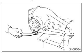
5) Remove the holder RH and LH with ST. ST 18630AA010 WRENCH
