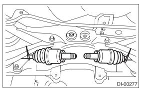
23) Remove the rear differential member plate from rear differential.
