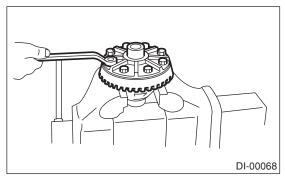
12) Drive out the pinion shaft lock pin from hypoid driven gear side.
