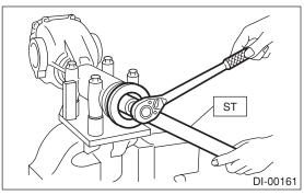
10) Assembling differential case Install the side gears and pinion mate gears, with their thrust washers and pinion mate shaft, into differential case.
