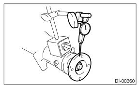
3) Set the gauge inside of the companion flange, and measure the runout.
