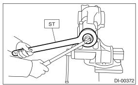
10) Install the hypoid driven gear on differential case.
