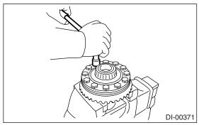
11) Support the companion flange with ST and remove self-locking nut.
