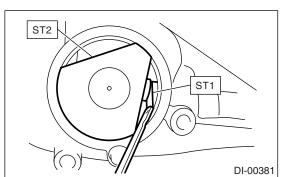
(4) Obtain the thickness of pinion height adjusting washer to be inserted from the following formula, and replace the temporarily installed washer with this one.
