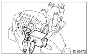
15) Draw a matching mark on both differential carrier and holder. Remove the holder side at a time. Replace in the original position after inserting an Oring and applying grease to threaded portion.
