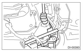
8) After inserting the rear differential stud bolt into rear crossmember bushing, lift up the transmission jack and align the rear differential to the height of rear differential.
