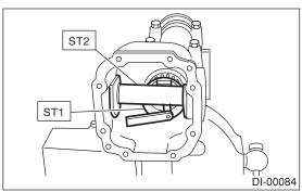
(3) Obtain the thickness of pinion height adjusting washer to be inserted from the following formula, and replace the temporarily installed washer with this one.
