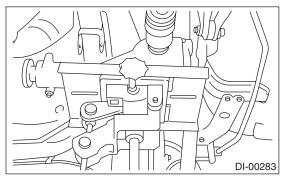
9) Tighten a new self-locking nut temporarily to rear crossmember.
