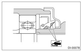
1) Adjusting preload for front and rear bearings: Adjust the bearing preload with collar and washer between front and rear bearings. Pinion height adjusting washer are not affected by this adjustment. The adjustment must be carried out without oil seal inserted.
