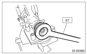
(2) Screw in the side holder LH until light contact is made with ST.
