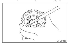
9) Extract the bearing cone with ST1, ST2 and ST3.
