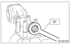
(2) Screw in the side holder LH until light contact is made with ST.
