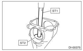
(2) Using the ST, install the front bearing race to the differential carrier.
