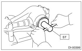
(3) Back off the side (hypoid driven gear side) holder approx.1 1/2 teeth of holder, and tighten the other side holder by approx. 2 teeth (approx. 1 1/2 + 1/2 teeth). [Back off amount of side (hypoid driven gear side) holder + 1/2 tooth.] This + 1/2 tooth gives preload.
