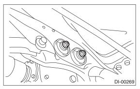
12) Remove the DOJ of rear drive shaft from rear differential.
