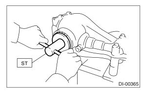
6) Pull out the differential case assembly from differential carrier.
