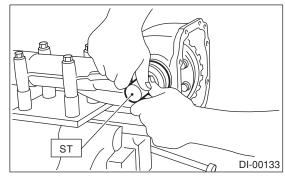
7) Pull out the differential case assembly from differential carrier.
