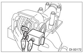
14) Draw a matching mark on both differential carrier and holder. Remove the holder side at a time. Replace in the original position after inserting an Oring and applying grease to threaded portion.
