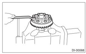
12) Press the side bearing into differential case using ST.
