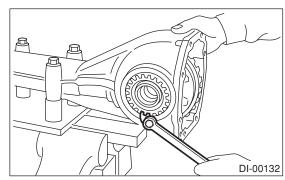
6) Remove the holder RH and LH with ST. ST 499785500 WRENCH ASSY
