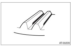
Corrective action: Reduce thickness of drive pinion height adjusting washer in order to bring drive pinion away from hypoid driven gear.
