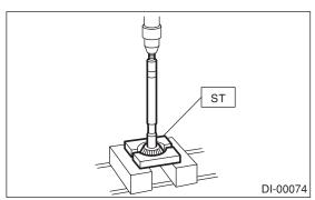
18) Remove the front oil seal from differential carrier using ST.
