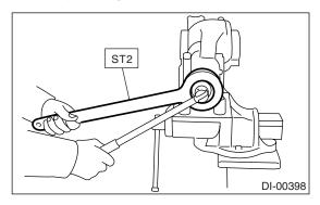
Drive pinion bearing preload
