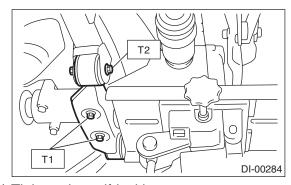
12) Tighten the self-locking nut.
