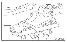
19) Lower the transmission jack stand after removing the rear differential stud bolt from rear crossmember. Rear drive shaft should not come into contact with lateral link bolt.
