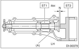
(A) Pinion height adjusting washer
