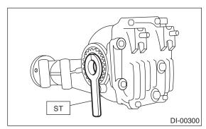
4) Insert the spline shaft until the spline portion comes inside the side oil seal.
