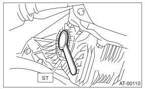
13) Install the ball joint of lower arm.
