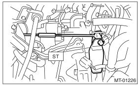
12) Remove the bolts which hold upper side of transmission to engine.
