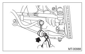
21) Remove the bolt securing ball joint of front arm to housing.
