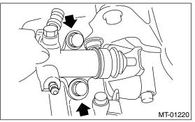
22) Connect the following connectors:(1) Transmission ground cable
