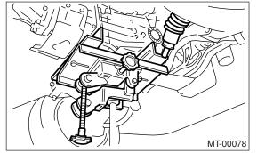
25) Remove the transmission rear crossmember from vehicle.
