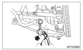
15) Install the gear shift rod and stay.
