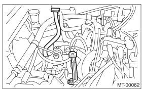
6) Remove the intercooler. (Turbo model) <Ref. to IN(H4DOTC)-12, REMOVAL, Intercooler.>
