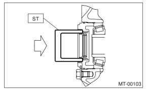
12) Install the front drive shaft into transmission.
