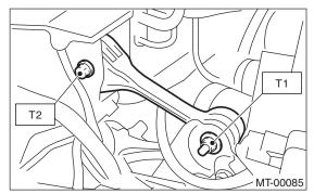
2) Install the air intake chamber and cleaner case. (Non-turbo model) <Ref. to IN(H4SO)-7, INSTAL-LATION, Air Cleaner Case.> <Ref. to IN(H4SO)-9, INSTALLATION, Air Intake Chamber.> 3) Install the intercooler. (Turbo model) <Ref. to IN(H4DOTC)-12, INSTALLATION, Intercooler.>
