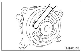
If the measurement is not within specification, select a suitable snap ring and replace it.
