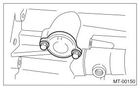
2) Install the ball, spring, washer and plug to transfer case.
