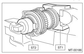
3) Remove the 5th-Rev sleeve & hub assembly, baulk ring, 5th drive gear & needle bearing.
