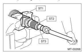
3) After removing the ST2, measure the starting torque using torque driver.
