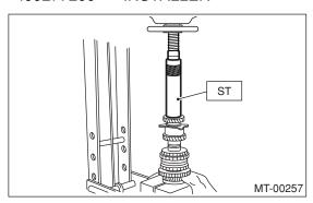
10) Install the lock washer. Install the lock nut and tighten to the specified torque using ST.
