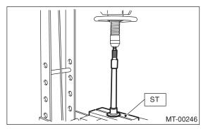
4) Unlock the caulking of lock nut. Remove the lock nut using ST1 and ST2.
