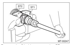
5) Remove the 5th driven gear using ST.
