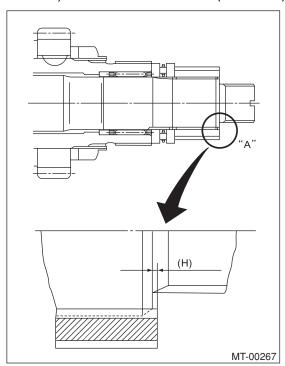
2) Using the ST1, ST2 and ST3, tighten new lock nut to the specified torque.
