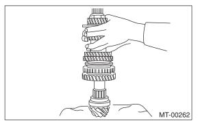
14) Install the drive pinion collar, needle bearing, adjusting washer No. 2, thrust bearing, adjusting washer No. 1 and differential bevel gear sleeve in this order.
