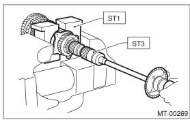
4) If the starting torque is not within the specified limit, select the adjusting washer No. 2 from following table, and recheck the starting torque.
