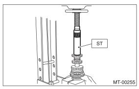
8) Install a set of roller bearings onto the driven shaft using ST and press.
