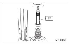
9) Position the woodruff key in groove on the rear of driven shaft. Install the 5th driven gear onto driven shaft using ST and press.
