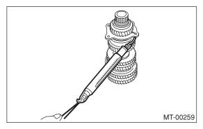
11) Install the roller bearing onto drive pinion.
