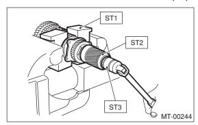
2) Draw out the drive pinion from driven shaft.
