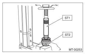
6) Install the 2nd driven gear, inner baulk ring, synchro cone and outer baulk ring, and insert onto driven shaft.
