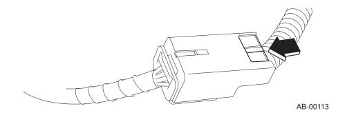
2) While the slide lock pressed in, disconnect the connector (A).
