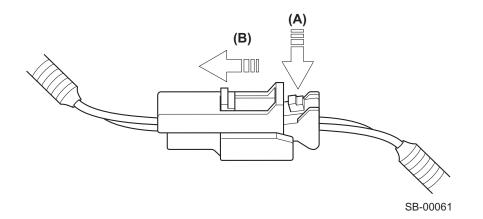
2) While the slide lock pulled and held (B), release the lock arm (C).
