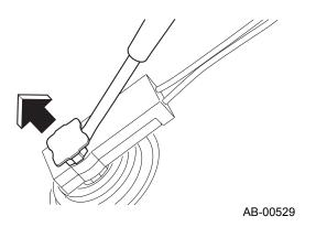
2) Pull the connector out from the airbag module.
