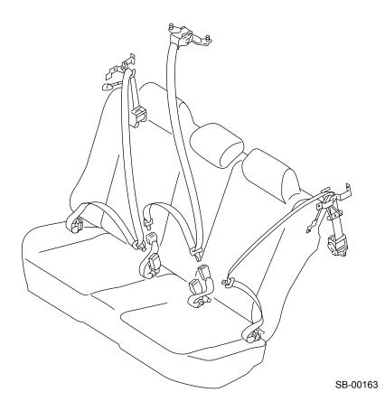
• Seat belts for the outer seats are provided with a new belt folding bracket at inside of the rear quarter trim to improve the appearance.
