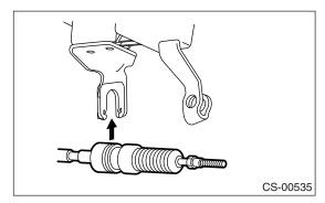
7) Shift the select lever to "N" range, and then adjust the select cable position. <Ref. to CS-26, AD-JUSTMENT, Select Cable.>
