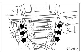
6) Disconnect the harness connector and antenna feeder cord, and then remove the audio.
