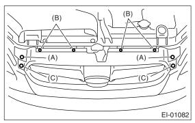
3) Pull lower side of the front grille forward, remove hooks (A), and then remove the front grille from vehicle body.
