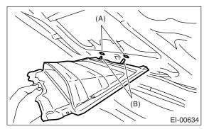
3) Install the front hood duct with the screws (A) and clip (B).
