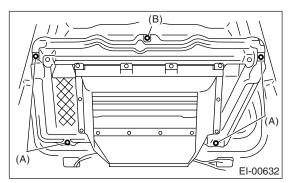
4) Loosen the nuts (A), remove the clip (B), and then remove the front hood grille.
