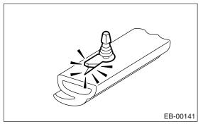
4) Remove the clip, and remove the cover cowl panel.
