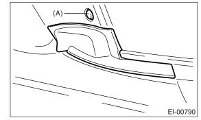
6) Remove the clips (A), and remove the cowl panel.
