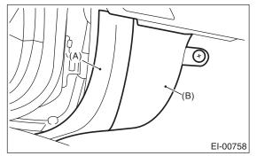
3) Remove the clips, and remove the instrument panel lower cover under.
