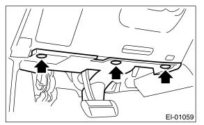
4) Loosen the screw (A), disconnect the connectors, and remove the instrument panel lower cover upper.
